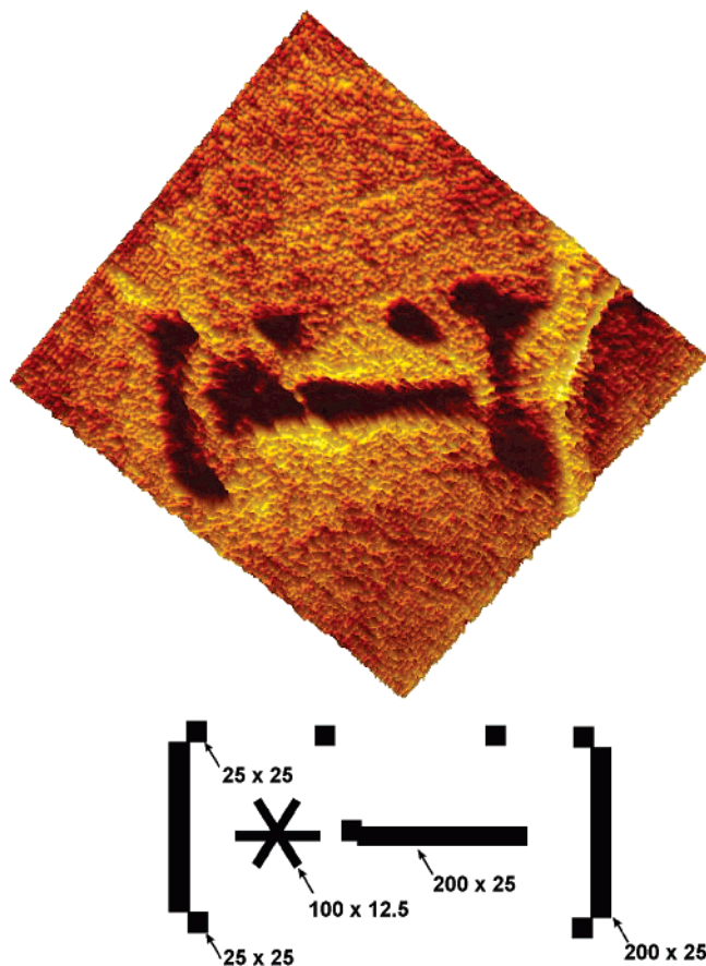
Figure 3. Heck-mediated aryl couplings patterned in the form of a Japanese emoticon. All dimensions are in nanometers.
